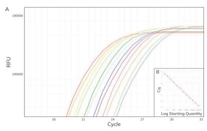
Reliable detection of 1.5-fold differences. Figure A. Amplification curves for assays of GAPDH in a dilution series of human reference cDNA (n=3). Assays were conducted using BioRad<sup>TM</sup> Sso Advanced SYBR Green Mix<sup>®</sup>. Figure B shows the standard curve obtained by plotting Cq values vs the amount of template DNA (copies/ $\mu$ I). R<sup>2</sup>=0.998, efficiency = 99.89%.
