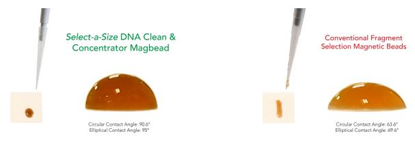
Reduced fluid surface adhesion for improved microliter pipetting. More consistent low volume magnetic bead transfers due to less reagent "stickiness" to pipet tips.
